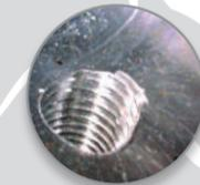
Burr in a cross hole in an ABS brake manifold viewed with a Hawkeye Pro Slim 7"
