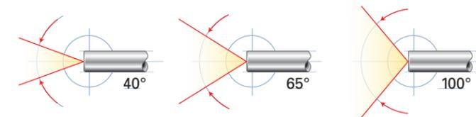
Most inspection situations need a "normal" objective lens (like a typical camera) with an angle of about 40°.
