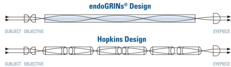
Our patented endoGRINs® gradient index lenses are the core technology of Hawkeye® Pro and Classic Rigid Borescopes. The elegant simplicity of the endoGRINs design gives excellent optical quality at a much lower cost than traditional alternatives, like the Hopkins design, which uses many expensive micro-lenses and optical glass rods.
