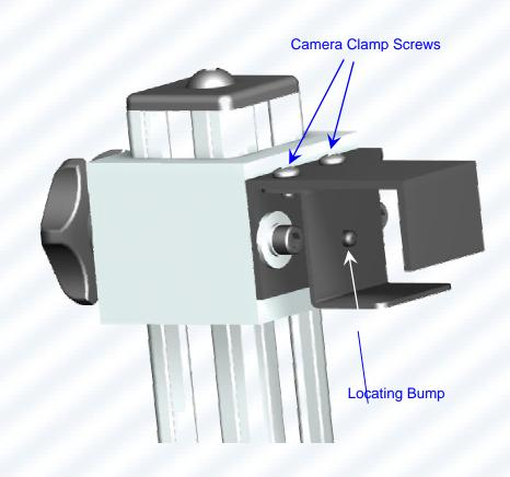
Loosen the Camera Clamp Screws 1 to 2 turns using a #2 Phillips screw driver. The screws are very short and will come out if turned too far. Be careful not to lose the screws.
