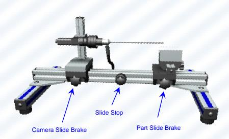
In either case, carefully position the slides so that the Borescope is at the maximum safe depth into the part. Tighten the brake on the slide chosen to be stationary. Then loosen the knob on the Slide Stop and move the stop until it is in contact with the slide chosen to be the moving slide. Tighten it down. Now as long as subsequent parts are mounted in the same position, the moving slide can be run until it contacts the stop without damaging the Borescope or the part.
