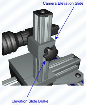
Camera height is adjusted by loosening the Elevation Slide Brake and raising or lowering the Camera Elevation Slide by hand. Tighten the brake to secure.
