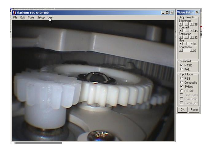
The other setting you can change is the image display and capture resolution. The maximum capture resolution is 640x480. To change the resolution, grab the lower right corner of the video window and drag it to resize to the resolution you want. If you want the software to restart with this setting, they select "Save Settings" under the File menu before you quit.
