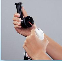
Clean the windows using a cotton swab dampened with Hawkeye lens cleaner, isopropyl alcohol or acetone.
