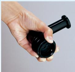
Push the borescope's eyecup into the housing and release the locking ring. Reverse to remove the borescope.
