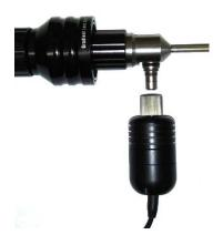
Plug the LXC-LED cable into the power jack on the bottom of the LXC.
