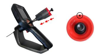
**2.** Replace the retaining nut and gently tighten by turning it in a clockwise direction.
