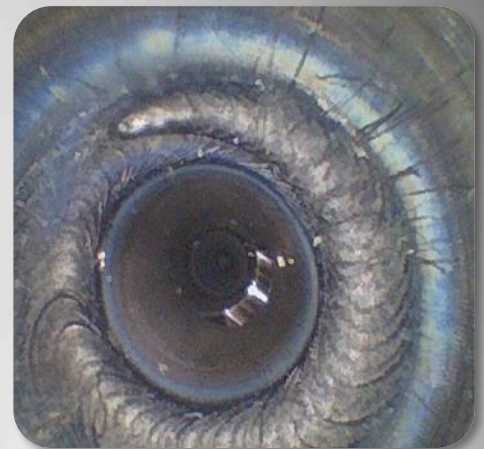
Stainless 1/3" Tube Orbital Weld Inspection using a .95mm VQ2 009 1000 NA
