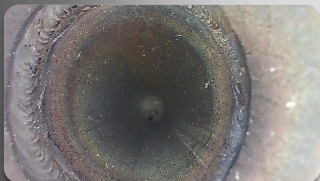
Orbital Weld Inspection Using a 4.5mm VQ2 045 1500 4D (Straight View)
