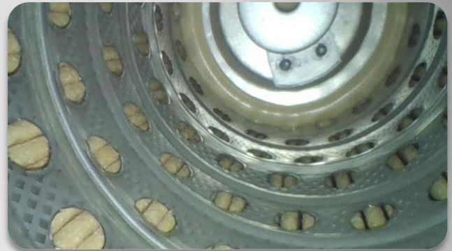
Lubrication Filter Inspection Using a 3.9mm VQ2 039 1500 4
