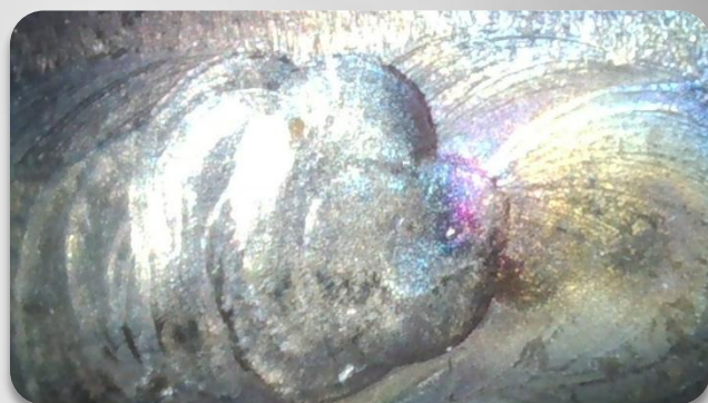
Orbital Weld Inspection Using a 4.5mm VQ2 045 1500 4D (Side View)
