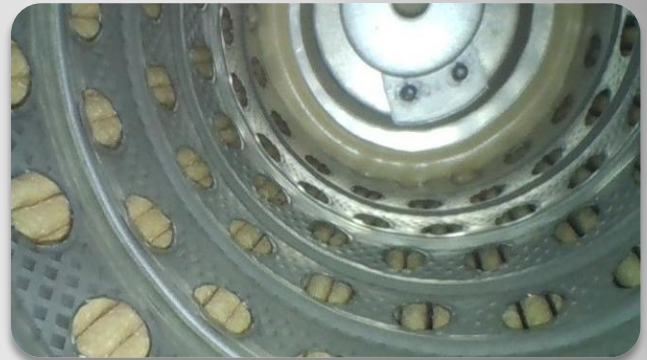
Lubrication Filter Inspection Using a 3.9mm VQ2 039 1500 4
