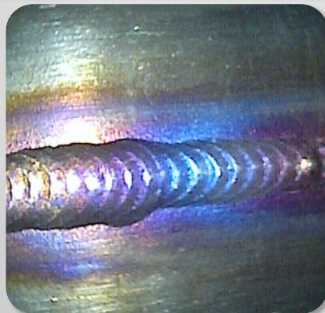
Orbital Weld using side view 2mm VQ2 020 1009 NL
